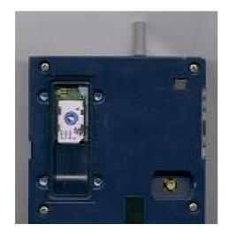
In the following procedure, it is assumed that a data SIM card has been inserted in the comm. Module slot as shown on the above picture, and the comm. Module has been plug to Z-Max unit again. Turn on both the Symbol and the Z-Max.
